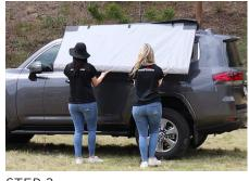
Undo the three Velcro straps around the car awning. Roll down the fabric/frame.
