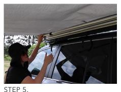
Person two can now unfold the two roof arms from the awning bracket.
