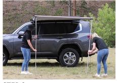
STEP 8. Lower both legs from the awning frame. Adjust to desirable height by twisting legs at the join.
