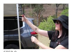
Secure the awning to the ground using the two tie-down straps and steel pins.
