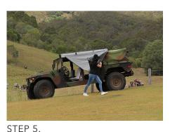
Using the now attached guide rope, start to open the awning. Walk the awning around the back of the car.
