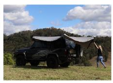
STEP 6. Walk the awning around the back of the car until complete expanded to 270°.
