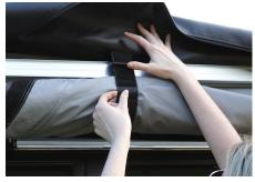
STEP 3. Undo the two Velcro straps around the car awning and roll down the fabric.
