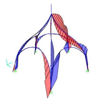
Max moment M\*= 0.11kNm 5.4.4 Max Bending Moment in minor axis due to critical load combination for columns
