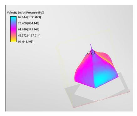
As it is illustrated, the wind tunnel simulator reveals the tent would undertake huge amount of pressure and suction in closed condition. Thus, due to enormous amount of deflection and weakness of the elements, the tent should never stand in closed condition.
