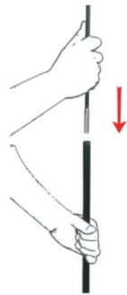
Insert the soft tube into the hole in the top of the connect pole
