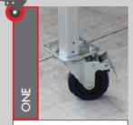
Ensure brakes are in the "on" position.
