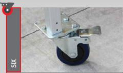
Set brakes to the "off" position (do not stand underneath).
