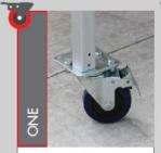
Ensure brakes are in the "on" position.
