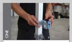
Attach half wall display connector to marquee leg. Repeat on other side.
