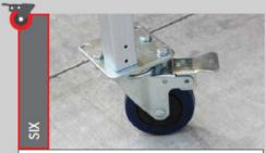
Set brakes to the "off" position (do not stand underneath).
