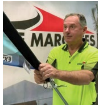
3. Applying even pressure pull the Banner Fabric to the base of the Banner Pole.
