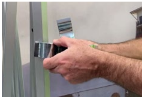
MARQUEE LEG CONNECTOR Position the Marquee Leg Connector in desired location and tighten until fitted.
