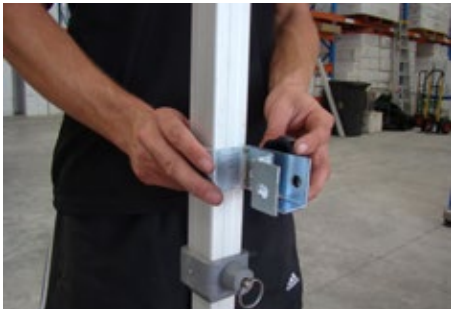
Attach half wall display connector to marquee leg. Repeat on other side.
