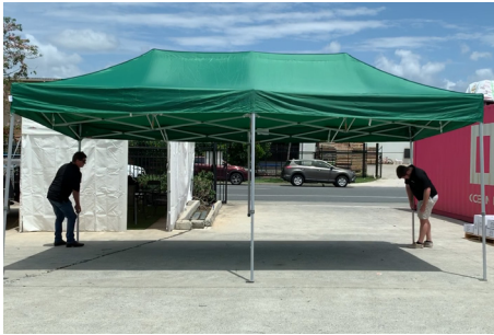
1. Push the lower leg button to fully retract the front middle leg. Repeat for front corner legs.
