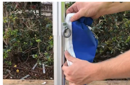
3. Insert the top of the Wall Strip Keda into the tracking of the Upper Leg of Canopy. (Hook facing inwards)
