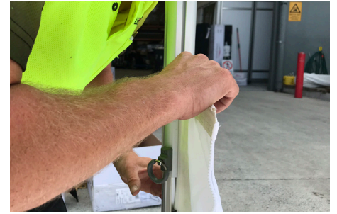
3. Insert the top section of the of the Wall Strip Keda into the tracking of the Upper Leg of Canopy.
