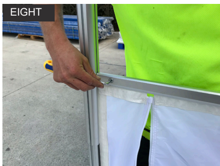
EIGHT Using the supplied tool, tighten the bolt lightly. Repeat on other side. Adjust the Half Wall Bar as need to be level and in desired position, tighten bolts to secure.
