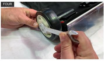
Spanner provided Tighten the bolt on the outside of wheel until tight.
