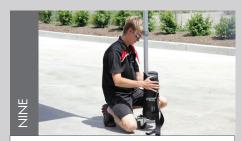
Fit sandbags or steel pins to anchor into position.
