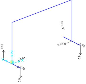
Max Reaction (Uplift)  $N^* = 0.9 \text{ kN}$
