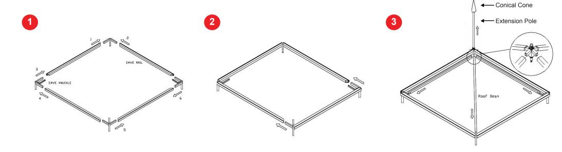
Lay out 4 x Eave Rails and 4 x Corner Connectors as above.
