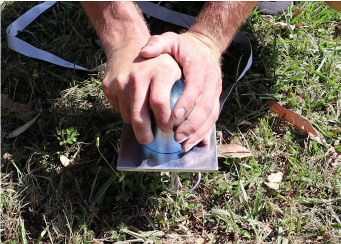
2. Push foot plate spike into the ground.
